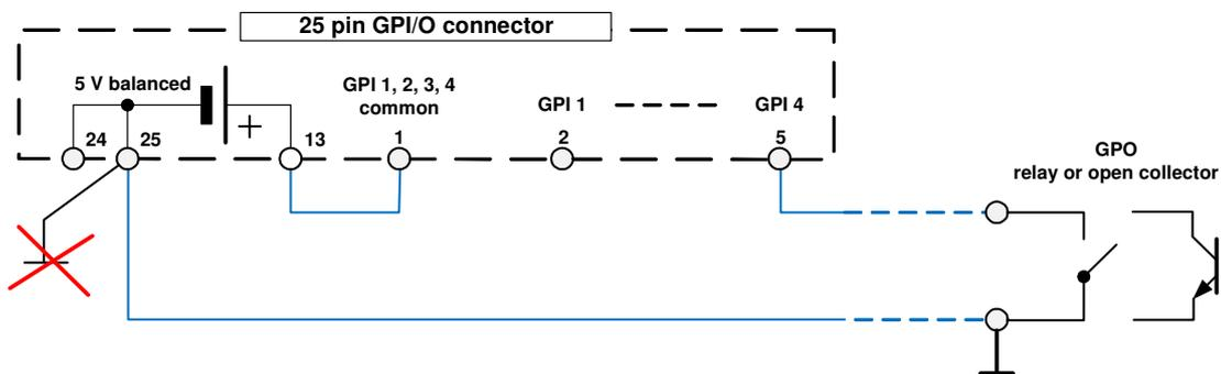
We strongly recommend providing a wire for ground connection instead of using the chassis common grounds of an installation.
