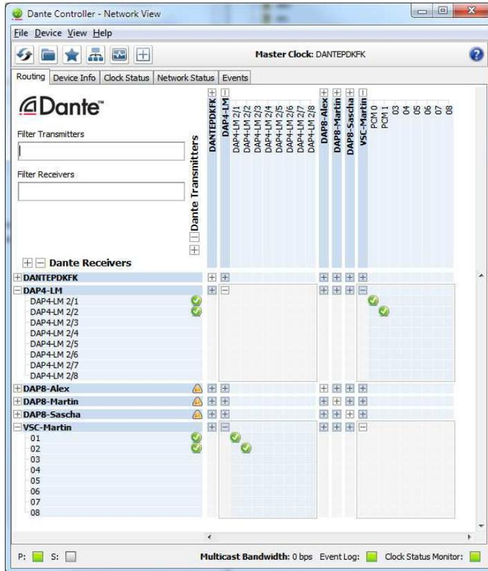
As an example you see here a "DAP4-LM" (name given by the Dante Controller) that has assigned the labels DAP-4 2/1 ... 2/8 for both the inputs and the outputs.
