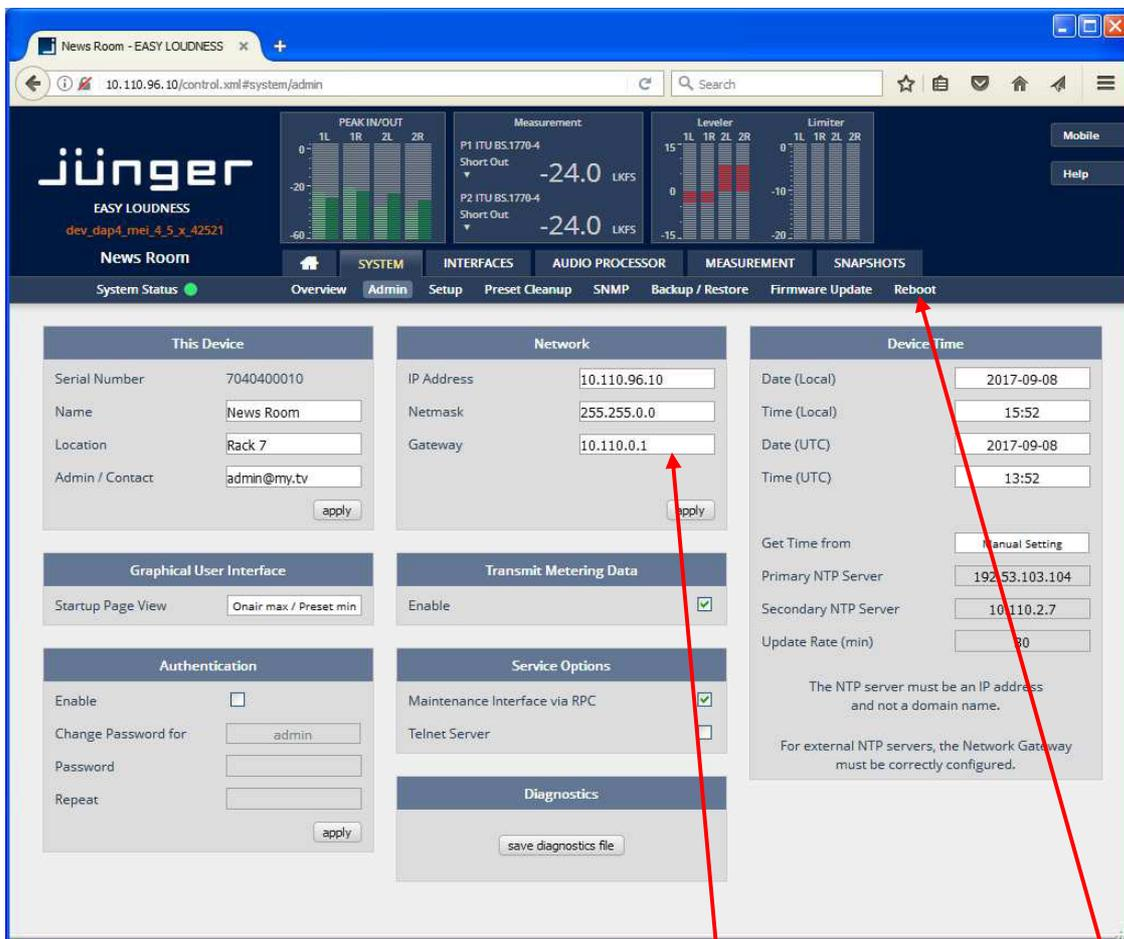
Enter the desired network configuration and press <apply> Afterwards you must reboot the **EASY LOUDNESS** in order to activate the new IP configuration.
