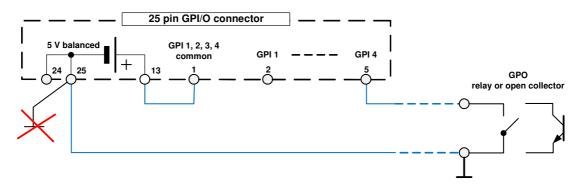
We strongly recommend providing a wire for ground connection instead of using the chassis common grounds of an installation.
