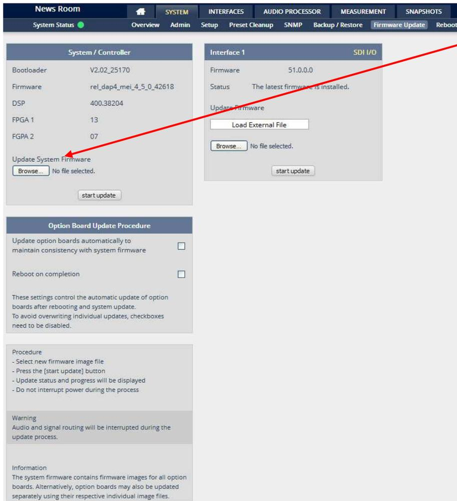
To update the **EASY LOUDNESS**, you must **<Browse ...>** to find the respective firmware file (which you have unzipped before) and press **<start update>**. After finishing the procedure the device will automatically reboot.
