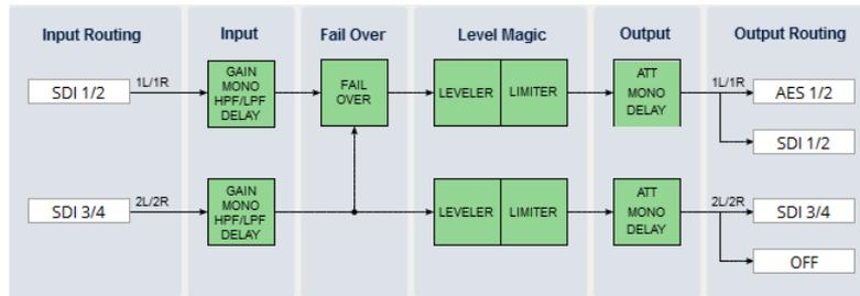
Above you see the various function blocks of the audio processor rendered by the **DSP** engine. Each function block has its representation in the GUI by individual tab sheets. You may simply click on the respective graphical area as an alternative way to navigate through the GUI.
