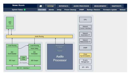
The graphical overview shows the main building blocks of the device including the options installed, in this example a SDI interface is placed into the interface slot (see rear view).
