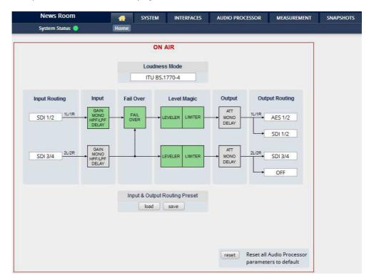
The processing blocks in use, which may be activated from their individual setup panes, will be indicated in green. I.e. blocks shown in grey are not activated by the user.
