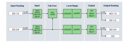
Above you see the various function blocks of the audio processor rendered by the **DSP** engine. Each function block has its representation in the GUI by individual tab sheets. You may simply click on the respective graphical area as an alternative way to navigate through the GUI.
