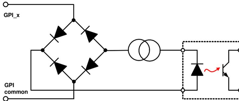
At the GPI input is a **bridge rectifier**, i.e. you do **not** need to care about the polarity of the input voltage. A **constant current source** in line with the **optical coupler** limits the current. You must simply provide a voltage in the range from 5 V to 30 V to activate a GPI.
