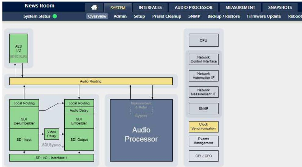
The graphical overview shows the main building blocks of the device including the options installed, in this example a SDI interface is placed into the interface slot (see rear view).
