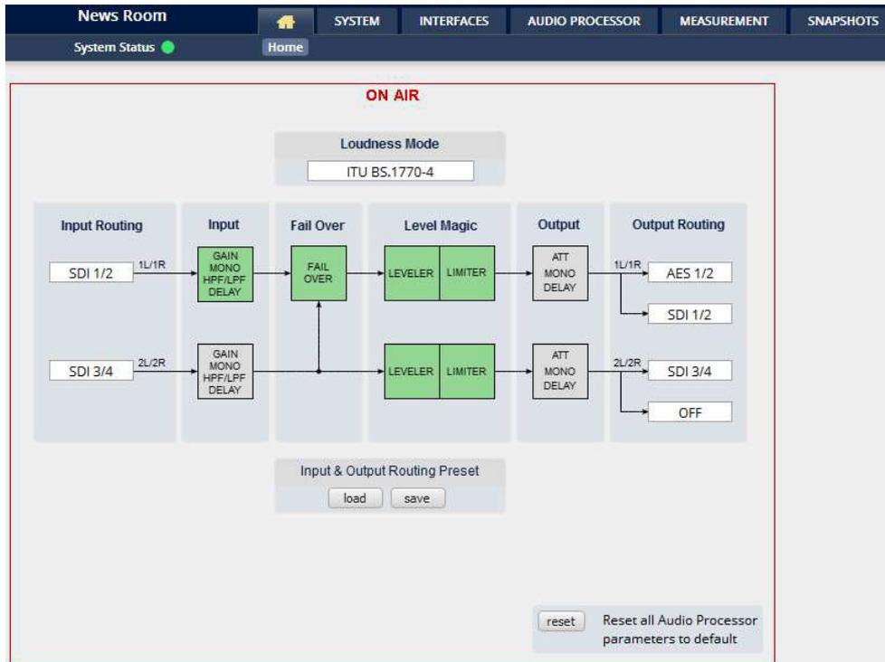
The processing blocks in use, which may be activated from their individual setup panes, will be indicated in green. I.e. blocks shown in grey are not activated by the user.
