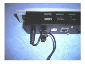
Important Note! There are older versions of the X\*AP RM<sub>1</sub> around which don't have a 5V input. These models must be powered via POE (power over Ethernet) either from a switch that has POE ports or from a POE wall power supply.
