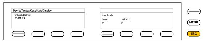
When you press a key of your choice the name of it will be displayed - in the example above, the **<BYPASS>** button. You can also check the rotary encoder by either turning the knob or pressing on it. If you turn the knob you will see the momentary value generated in linear and ballistic values. Pressing on the knob will show the name **ENTER** in the left display.
