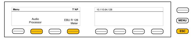
The Audio Processor has the following functions available which you can reach via the F-Keys: #1<Input> #2<Upmix> #3<Equalizer> #4<Spectral Signature>
