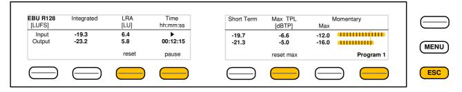
In this case the <F-Keys> will control the program based loudness measurement process defined by EBUR128. The display represents the measurements of Integrated- / Short Term- and Momentary-Loudness as well as the LRA (Loudness Range) [LU] and Max TPL [dBTP], the Maximum True Peak level.
