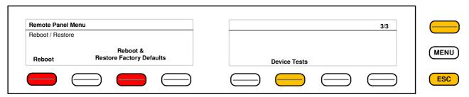
Page three allows you to reboot or restore of factory defaults. It also offers testing the device. **X\*AP RM1** remote panel LEDs, buttons and the rotary knob. Pressing the Device Test button opens up further menus to test the respective items.
