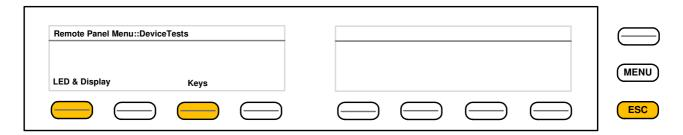
Pressing <LED & Display> lets you check the bar graph and status LEDs basic colors:
