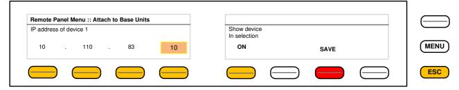
Same procedure: Set up the IP address of the device you are about to attach.
