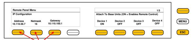
You may press the respective **F-Keys** and a separate window will appear for comfortable set-up of the respective part of the IP configuration.
