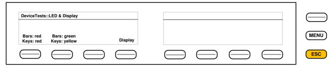
All bar graph and key LEDs must light in the respective color. Pressing the **<Display>** button will turn on both display windows in amber color. You will return by pressing the **<ESC>** button.
