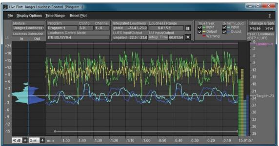
The tool keeps all data gathered from the selected processing channel in the PC RAM. This allows you to change the time scale by selecting it from the pull down menu **<u>Time Range</u>** or by the pull down box on the bottom left side: 2 min **u** at any time you like. The tool keeps data for 2 hours in the RAM, for both the input and the output. After that it starts cycling the data in FIFO (first in first out) style.
