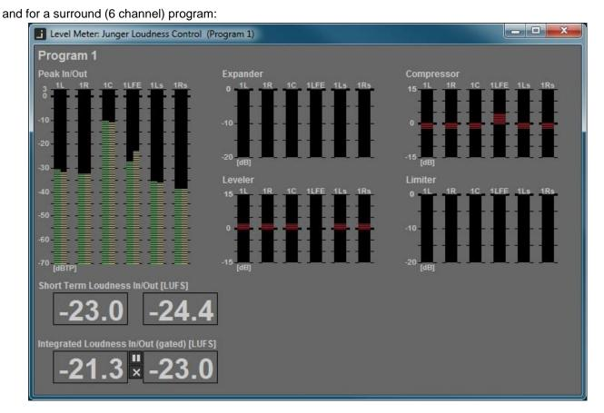
It shows the input vs. output peak level, the limiter as well as the leveller gain reduction plus Short Term and Integrated Loudness.
