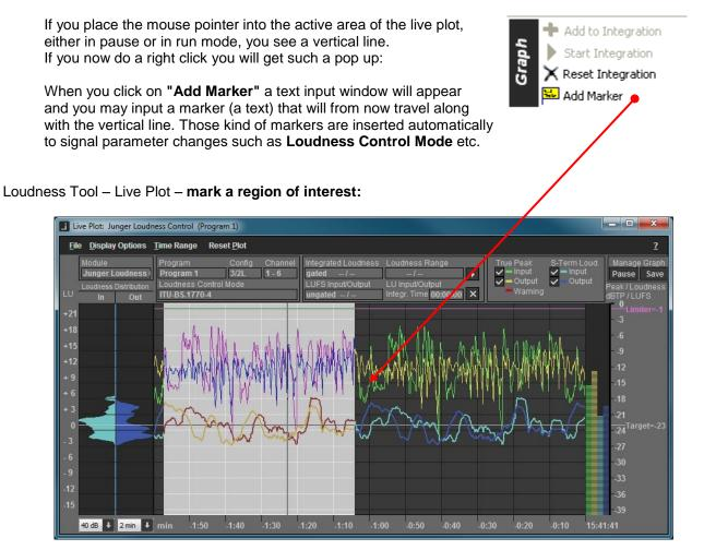
You must place the mouse inside the plot window, click the left button and drag the mouse over the region of interest. When you release the button, the region will be highlighted and a small option pop up opens:
